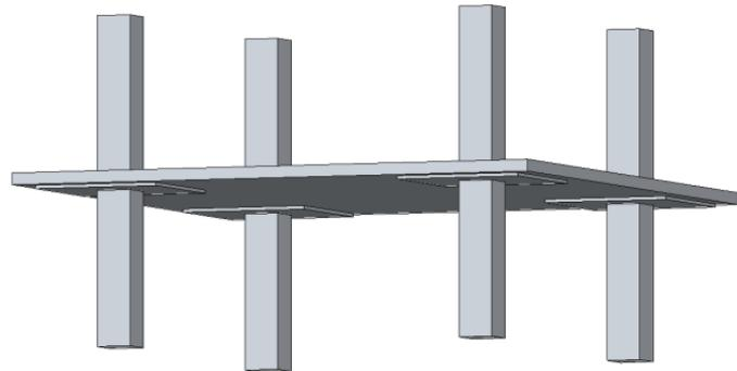
Figure 5: Flat Slab Floor System
