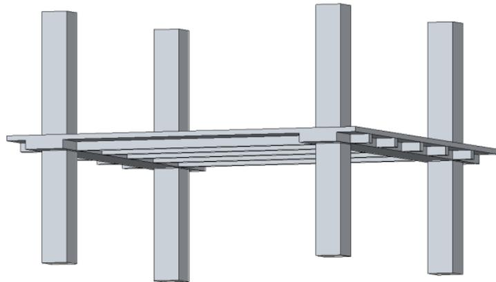
Figure 6: One-way Joist Floor System
