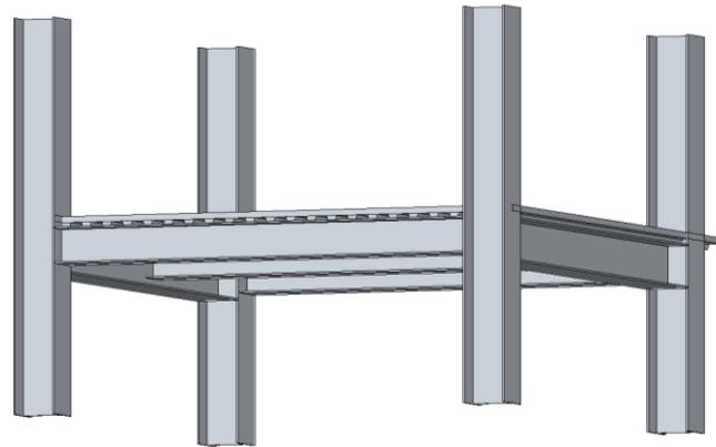
Figure 3: Existing Floor System: Concrete on metal deck with steel framing
