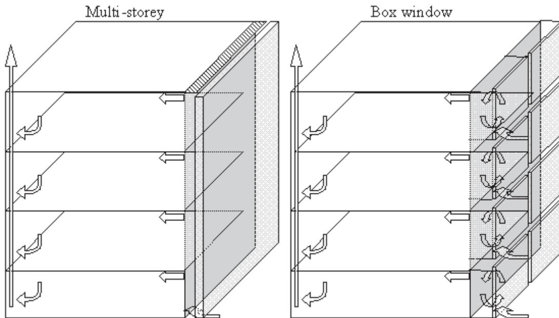
Figure 8: Double skin façade as individual supply of preheated air, image from Harris Poirazis: *Double Skin Facades*
