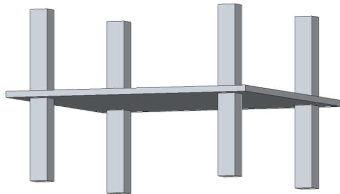
Figure 4: Flat Plate Floor System
