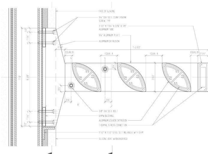
Figure 13: Exterior Louver Detail
