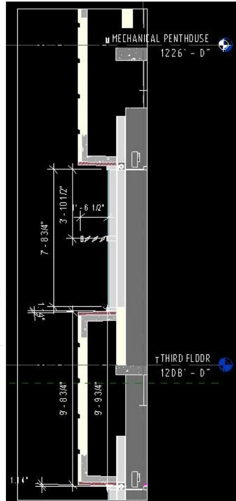
Figure 14: Typical Exterior Wall Section
